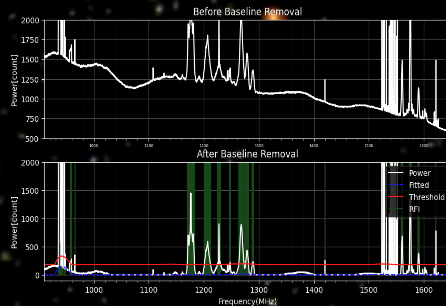
Figure 2. A comparison of a MeerKAT test data taken on 2020-03-26 before and after baseline removal
