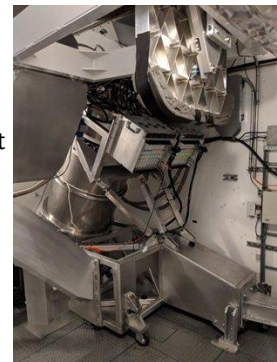
(Top) Grating spectrometer. There are 16 feed horns spanning spatially, and 60 spectral channels.
